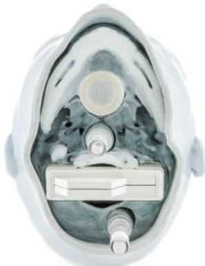
Reference PseudoPatient™ phantoms are accompanied by the RTsafe-provided multi-target SRS package modeling a reference set of seven targets and organs at risk (OARs) for a realistic multiple metastases case. Alternatively, feel free to create your own set of targets and OARs, simulating a challenging SRS/SRT case.
