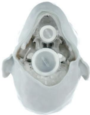
**Reference PseudoPatient™ MI:** Reusable multi-insert head phantom which can be filled with water as a tissue equivalent material. The phantom is properly machined to accommodate two interchangeable inserts for point dosimeters at specific locations within the brain and a film holder located at a central coronal plane. Absolute real-time point and 2D film dose measurements can be performed by the end-user.
