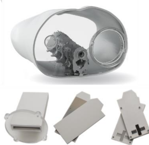
Figure 1: The RTsafe SBRT phantom, along with the appropriate inserts to accommodate Gafchromic EBT film and OSL dosimeters.
